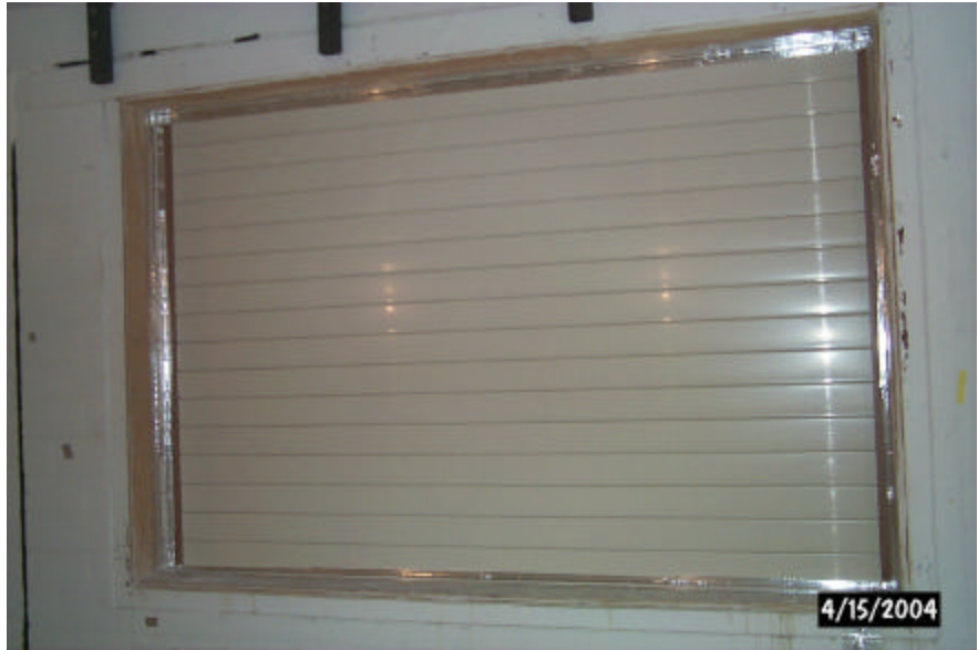
Figure 1: The specimen B3410-1 installed in the wall test frame.
